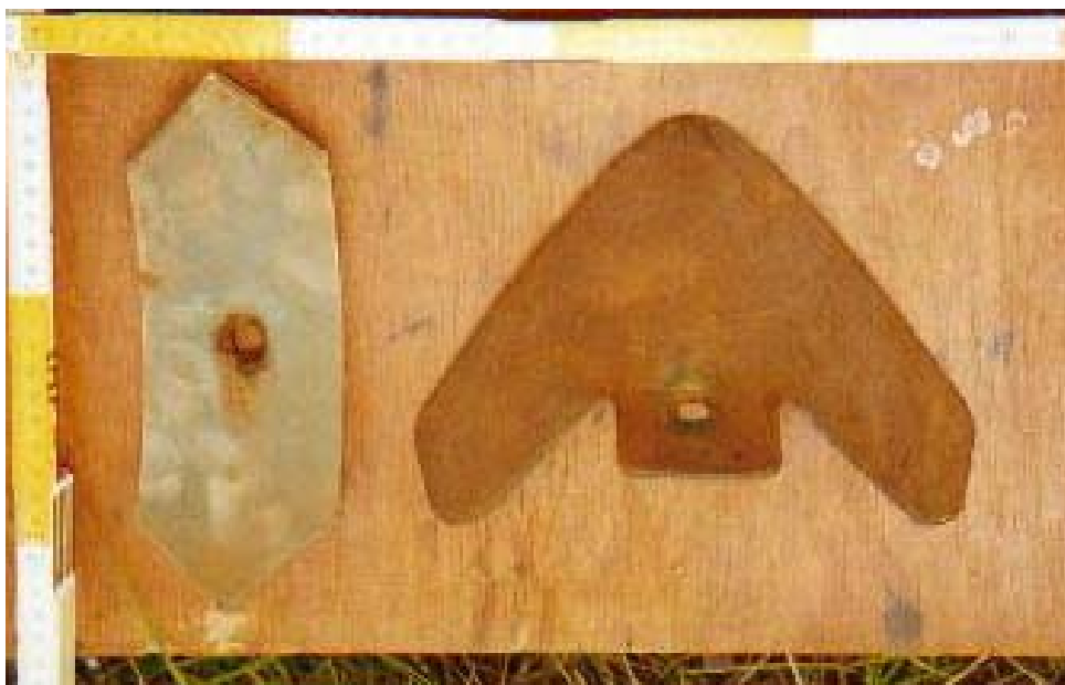
Fig 1 Reversible (left) and duck foot (right) tines
