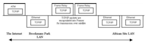
Frames are sent over Virtual Circuits. These circuits are connections between locations on the Frame Relay system. Data Link Connection Identifiers (DLCIs) are used for addressing. A DLCI is a 10-bit address that identifies a particular permanent virtual circuit, a bit like an IP address identifies a device in TCP/IP networks, except that a DLCI identifies a link, while an IP address identifies a device.
