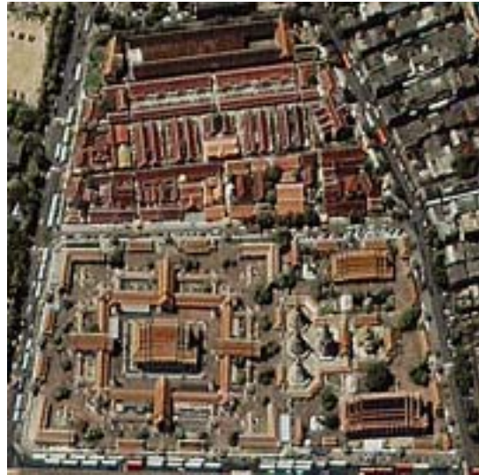
Figure 2.1 Vertical aerial photograph and vertical satellite image illustrating radial distortion
