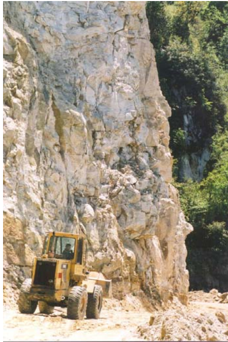
Highly fractured rock mass without continuous joint surfaces.
