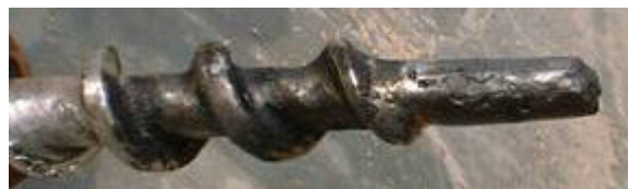
Plate-4.7 Worn out Traditional Screw after 9 Hours of Operation
