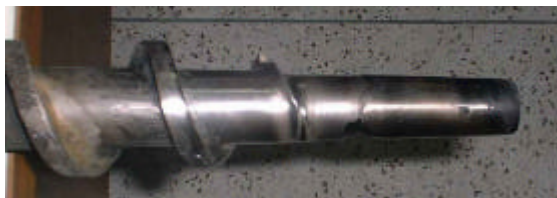
Plate-4.6 Worn Out New Screw after 16 Hours of Operation
