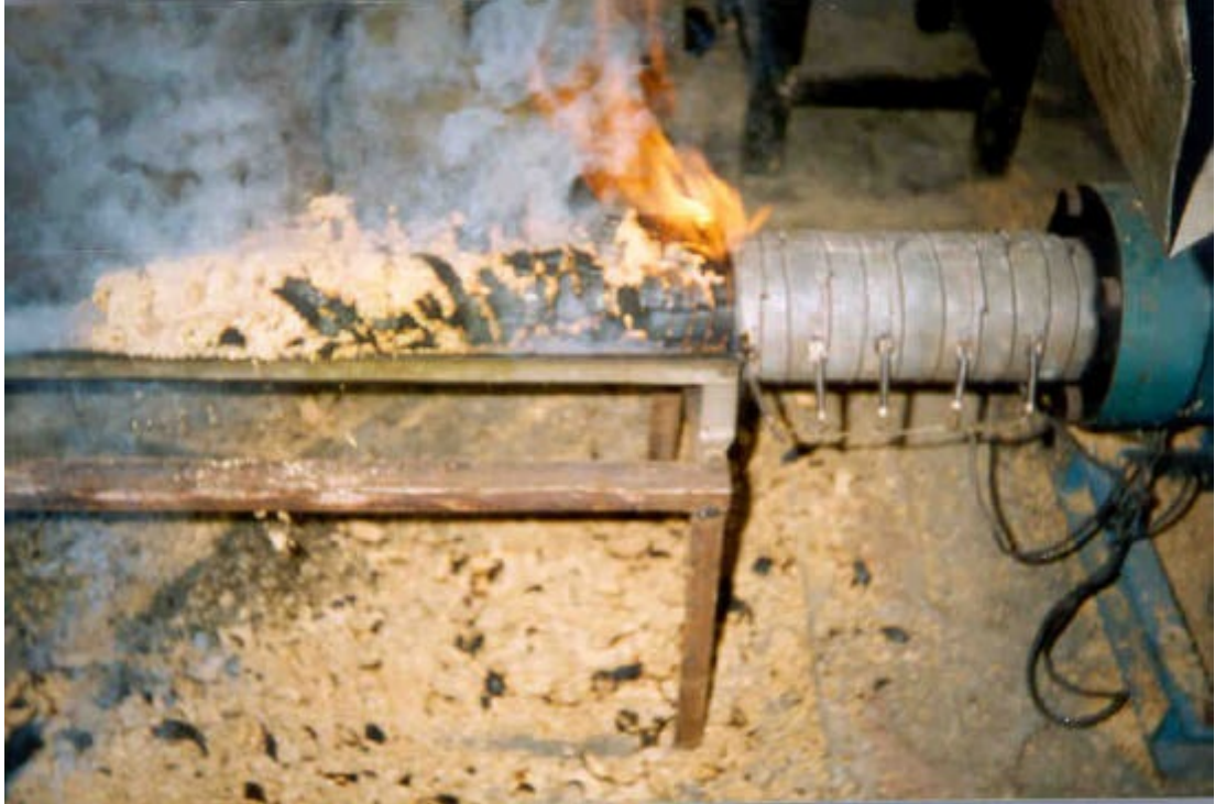
Barrel heating with electricity
