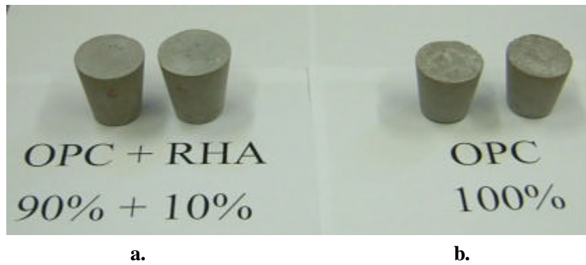
Figure 6 Specimen Blocks made from a. Specimen Blocks made from 90% OPC+ 10% RHA, b. 100% OPC.
