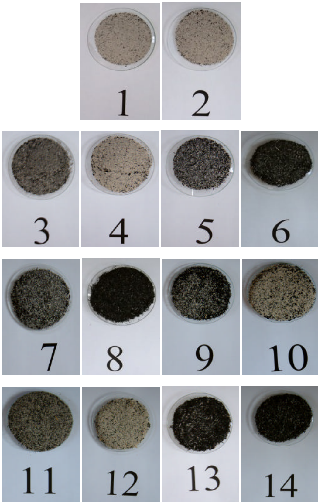
Figure 2. Photographs of Rice Husk Ash Samples from Bangladesh
