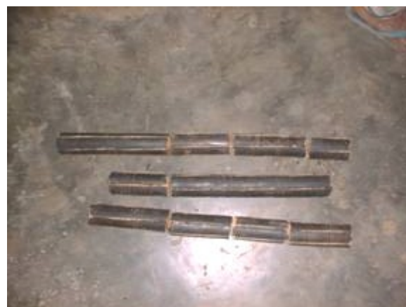
Plate-4.3 Broken Briquette Produced by New Screw after 16 hrs
