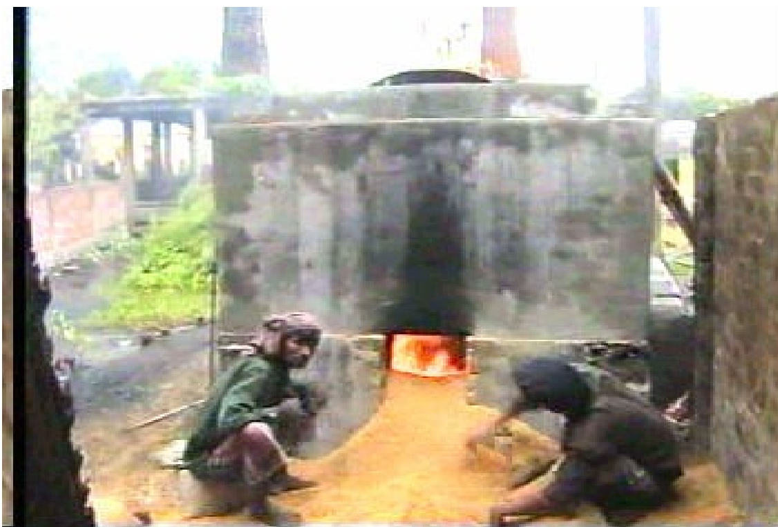
Plate 3.2 View of the Furnace Showing the Fuel Inlet Port and Furnace in Operation
