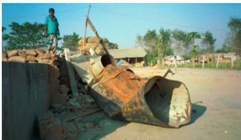
Plate 5.1 Showing the Aftermath of a Boiler Explosion
