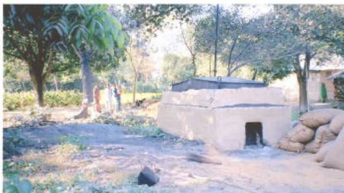
Plate 2.3 Rectangular Box Boiler
