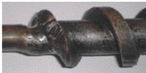
Deteriorated part of the screw
