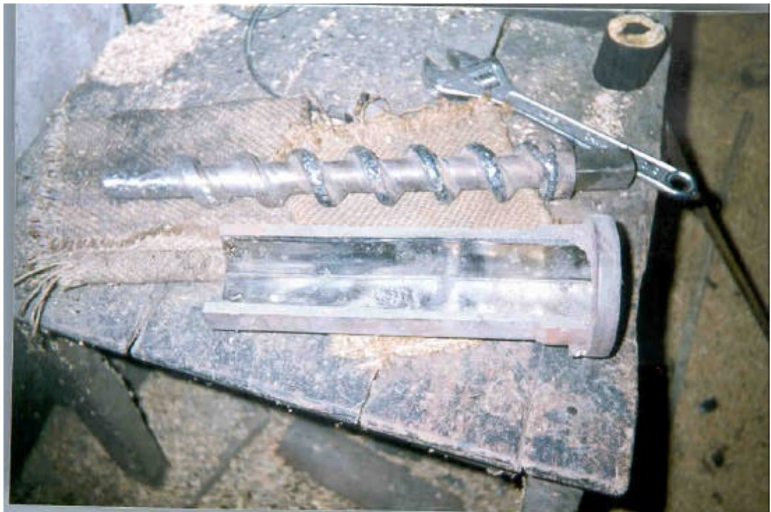
Worn out screw and barrel
