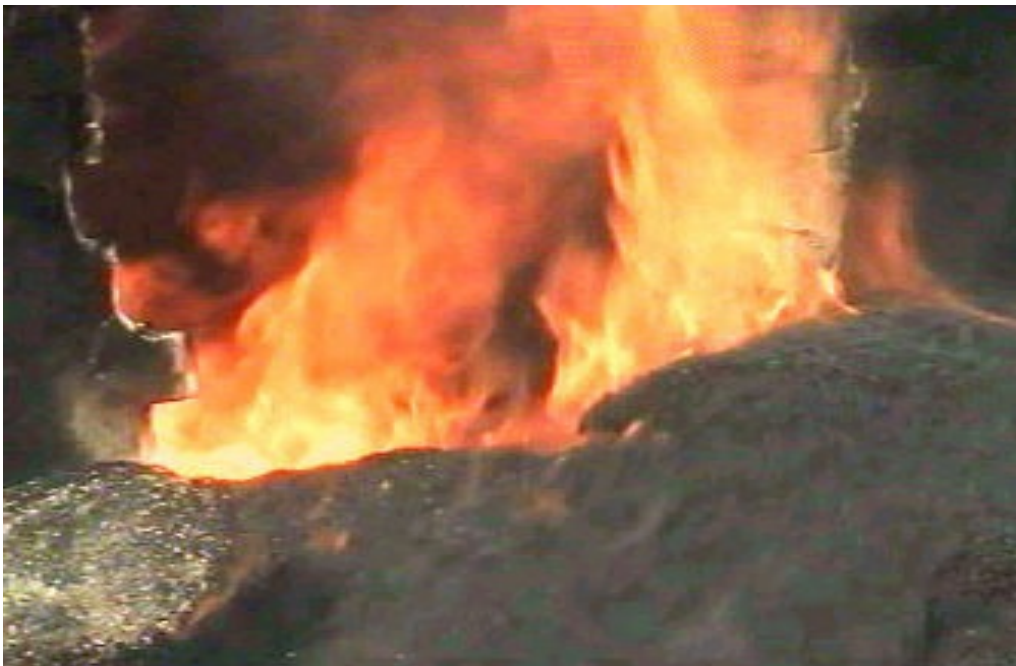
Heat Loss from Side Port and Ash Port
