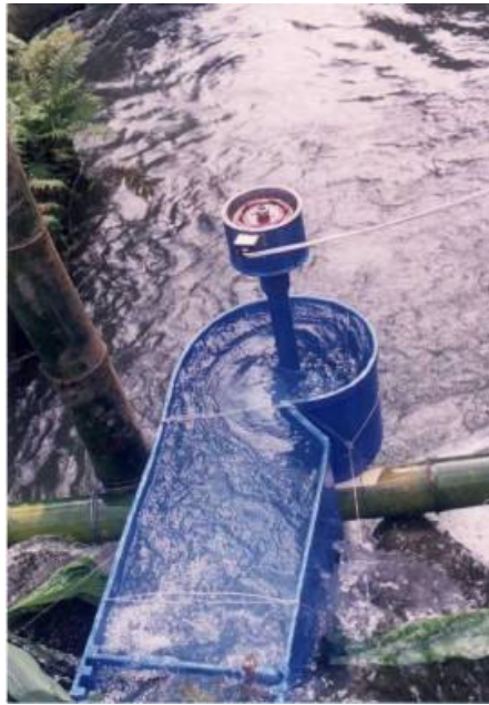
Figure 2 – Vietnamese 200 W low-head pico-hydro 'propeller' unit in the Philippines
