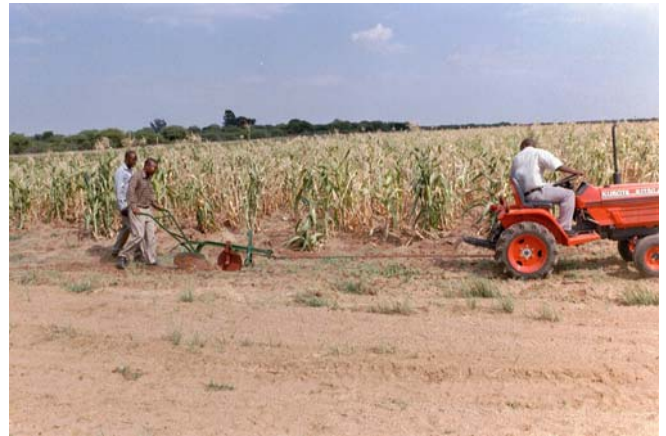
Figures 1.3, 1.4. The plough with trench wall cutting attachment. Unfortunately, the soil was too dry for effective testing on this occasion.
