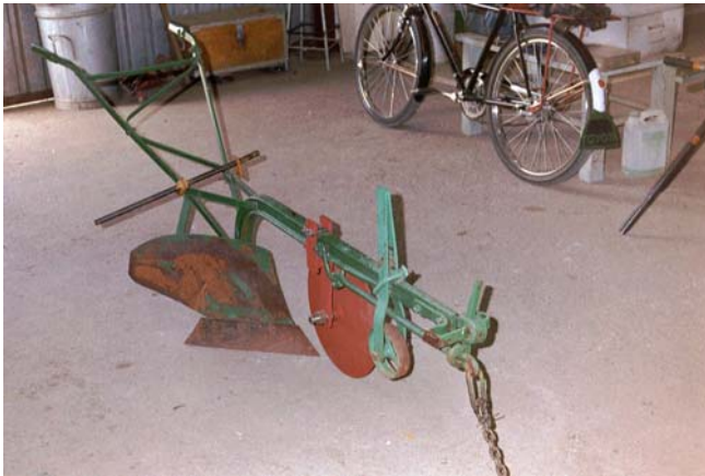
Figures 1.3, 1.4. The plough with trench wall cutting attachment. Unfortunately, the soil was too dry for effective testing on this occasion.
