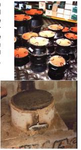
**LPG cylinders and bottles**: LPG is transported and stored as a compressed liquid in canisters ranging in size between 3kg and 50kg or larger. For household use, gas is conveyed via simple regulators and pipes to stoves or lamps, which are specially designed for LPG use.
