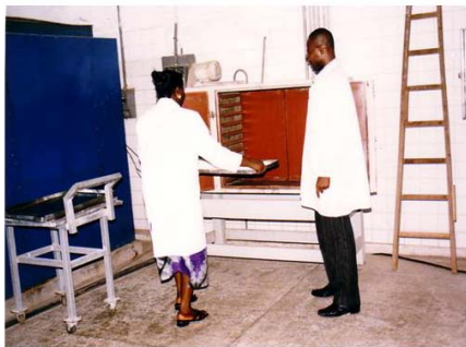
A workshop participant placing a tray full of disintegrated cassava in a cabinet dryer.
