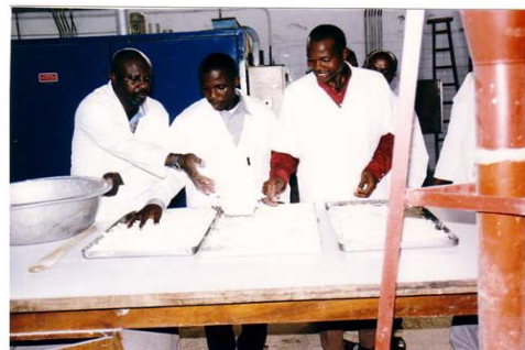
Workshop participants spreading disintegrated cassava mash in readiness for drying.
