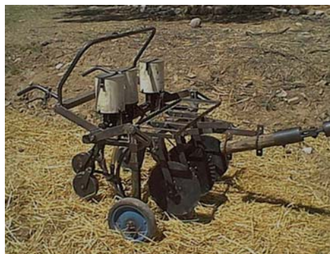
Figure 5. Direct seeder for small cereals designed to be pulled by a pair of oxen. Bolivia.
