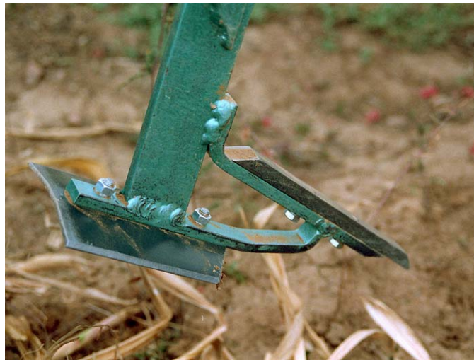
Figure 4. Wing-tined chisel plow for more efficient soil bursting during vertical tillage.
