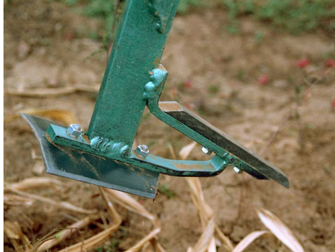
Figure 5. Wing-tined chisel plow for more efficient soil bursting during vertical tillage.
