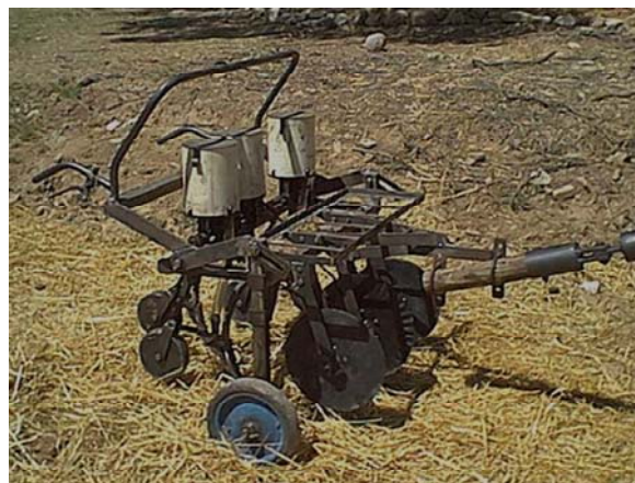
Figure 6. Direct seeder for small cereals designed to be pulled by a pair of oxen. Bolivia.
