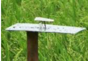
Figure 1c Sticky plate trap
