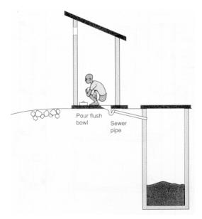
Advantages: Provided that the groundwater is deep enough, leach pits provide a simple mean of disposing of black water in a way that harms neither the environment nor public health.
