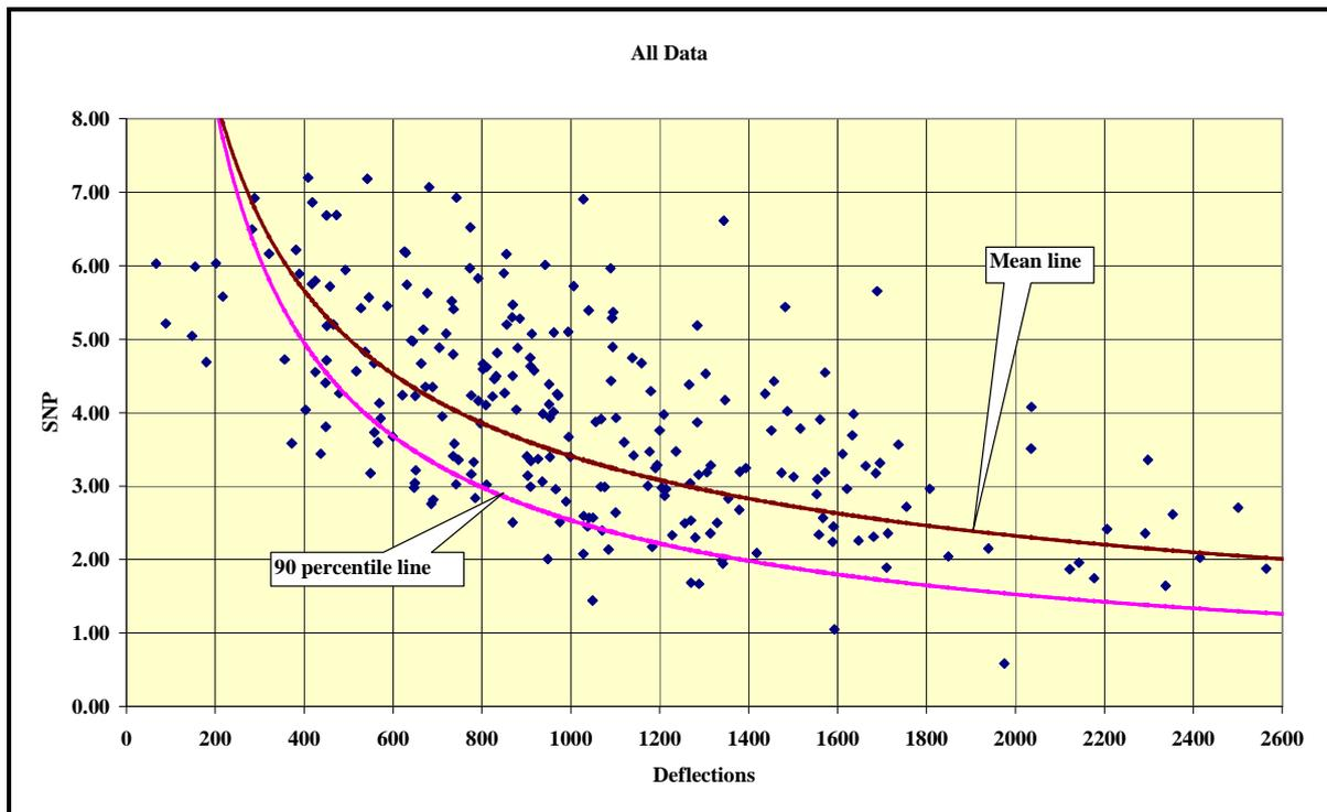
**Figure 3.1 Relationship between deflection and structural number**
