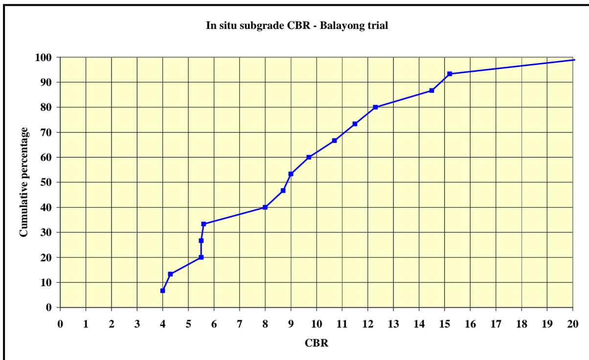
Figure 4.2 Distribution of subgrade CBR's for Balayong trial
