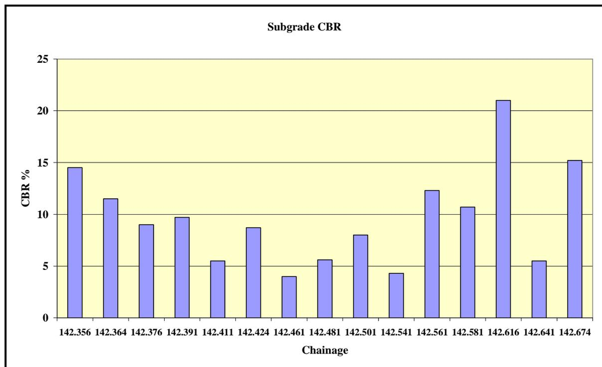
**Figure 4.1 Subgrade strength distribution along the site**
