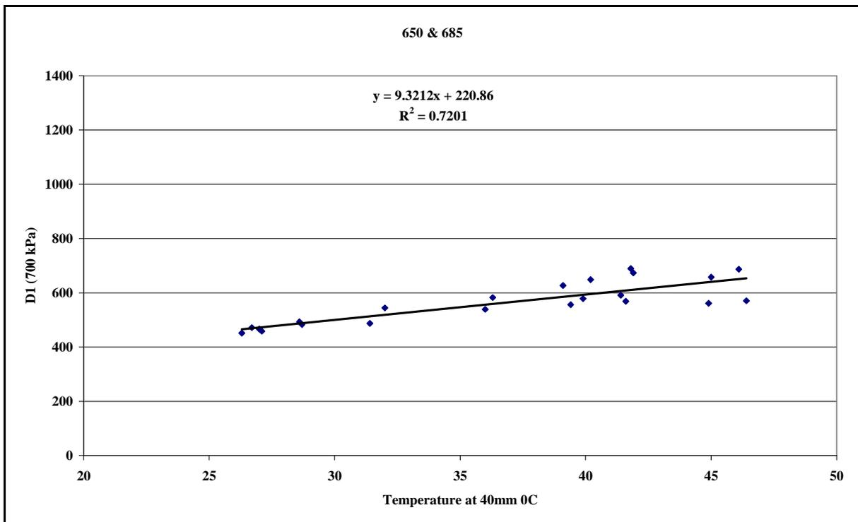
**Figure E5 Central deflection at chainage 141+650 plus 141+ 685**
