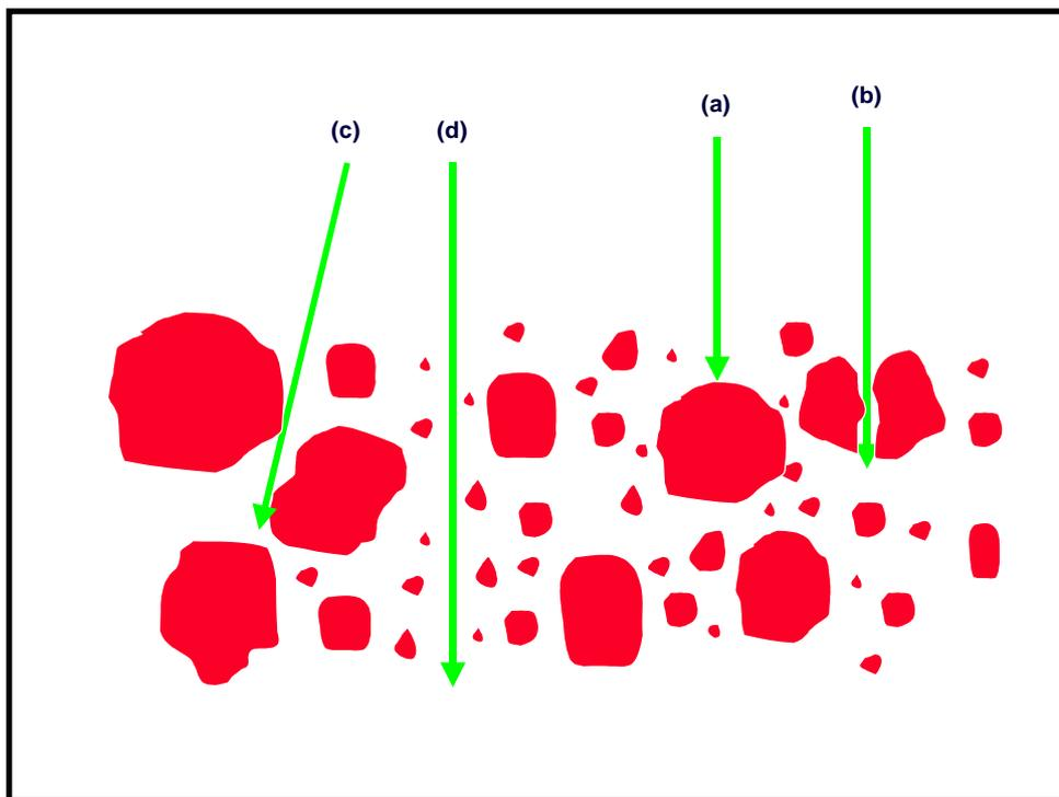
**Figure F1. Typical DCP effects with large stones**
