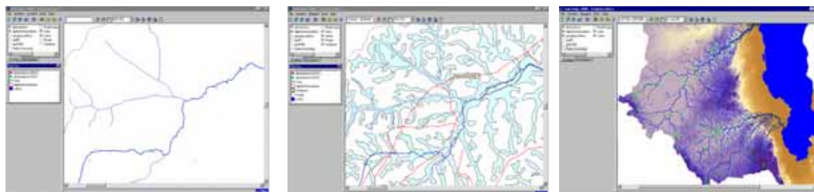
Figure 4.12 GIS interface showing river stretches and abstractions before and after the addition of contextual layer (wetlands and roads), and a picture of the underlying topography
