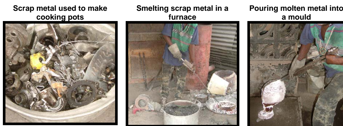
Figure 10: Cooking pots being manufactured by informal a foundry
