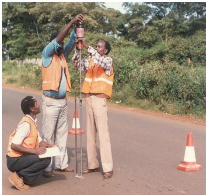
Fig. 2 Dynamic Cone Penetrometer in operation
