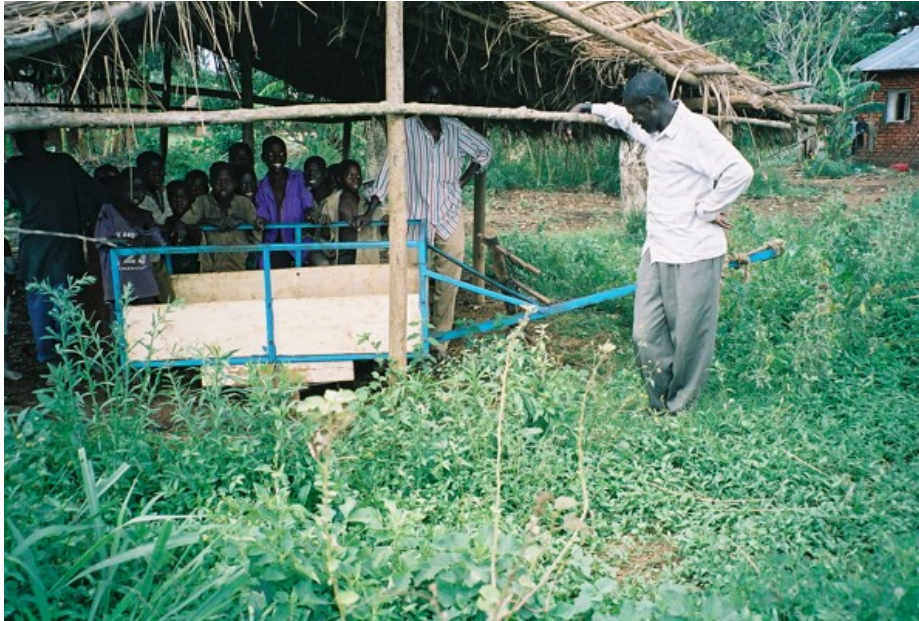
Fig A3.1 Donkey cart with wheels removed for repair (replacing tubeless tyres with tyres having tubes)
