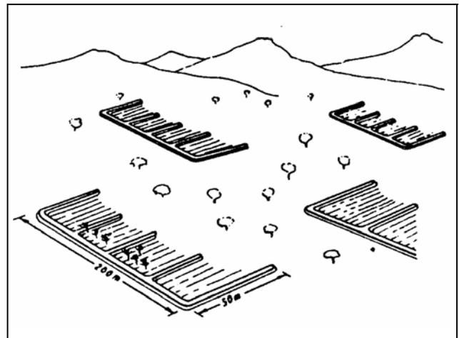
Figure 6: Examples of hill sheet flow RWH
