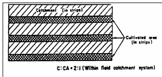
Figure 4:RWH with Strip Catchment Tillage
