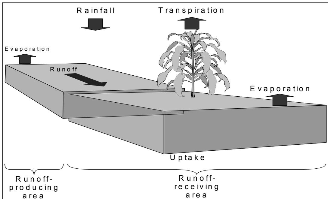
Figure 2: The hydrological components of a conceptual rainwater harvesting system.
