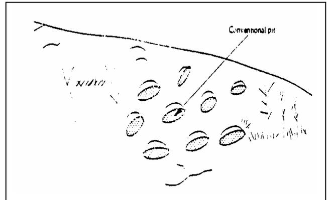
Figure 3: Layout of Pitting RWH
