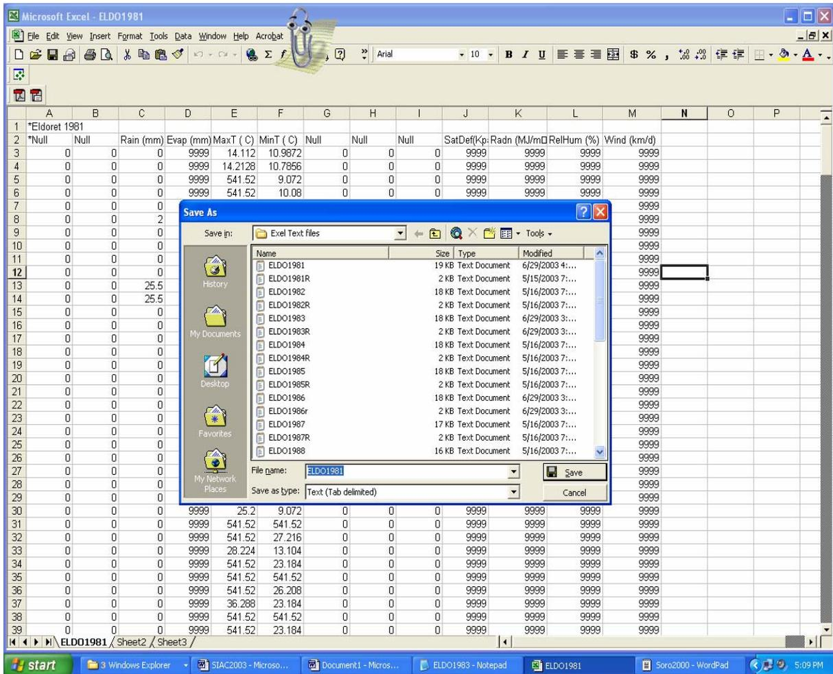
Figure 29: Saving data in Text Format
