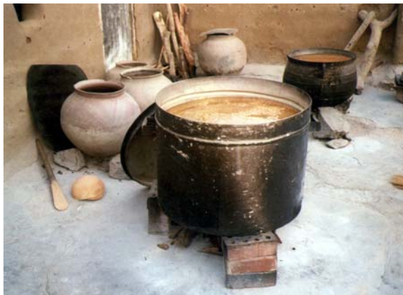
The new parboiling vessel holds 100kg paddy
