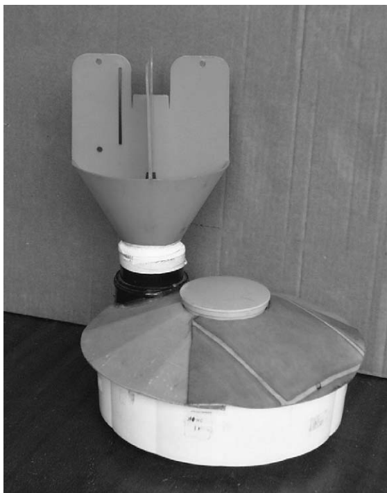
Fig. 2. Assembled pheromone-baited flight trap for segregating catch with time.
