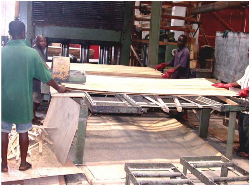
Glue-coated veneer sheets ready to go to the pressing machine.
