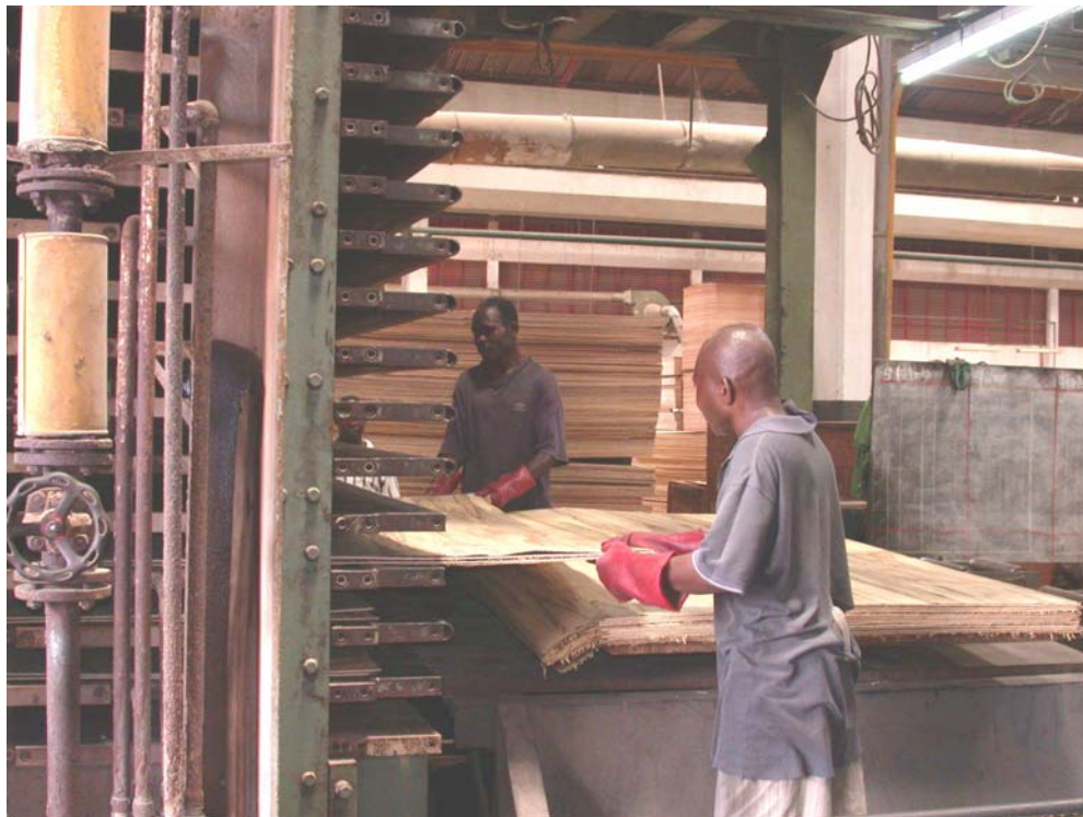
Glue-coated veneer sheets being packed into pressing machine.
