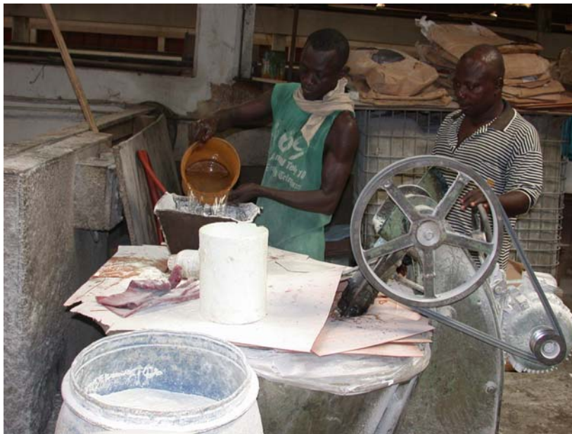
Mill trials: Formulation of plywood adhesive with cassava flour. Water being poured into the mixing machine.
