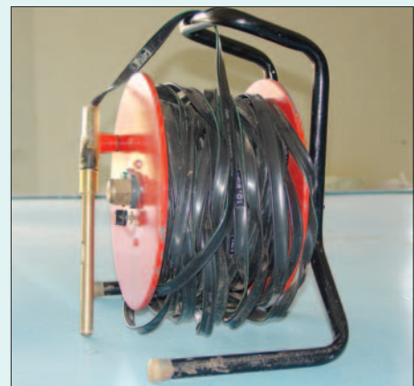
Ground water level measuring device
