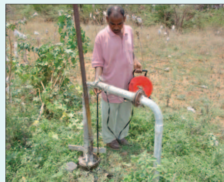
Farmer measuring water level in the bore-well using the device
