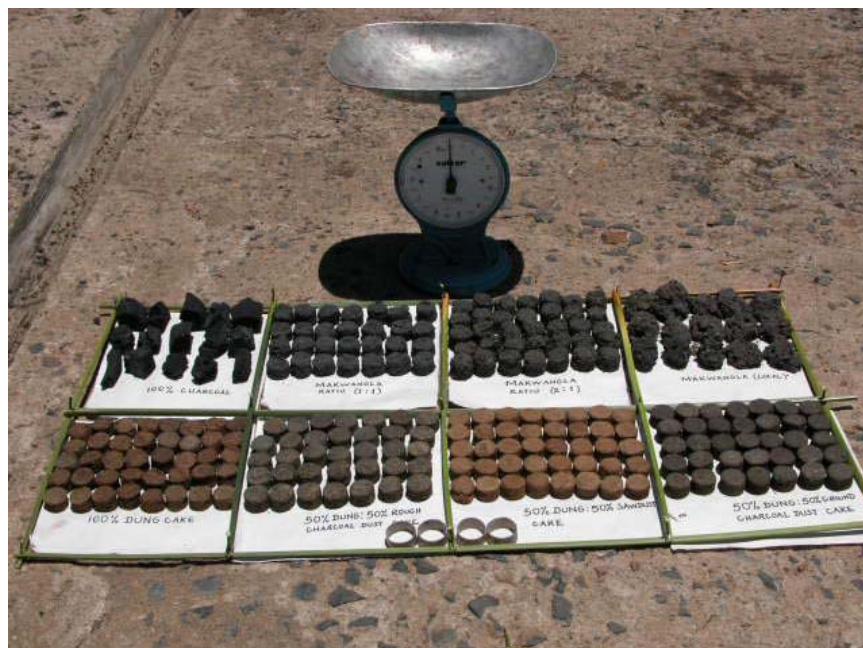
Figure 2. A picture showing eight types of fuel cakes made using pvc pipe as a mould (front of the picture) ready for burning test.
