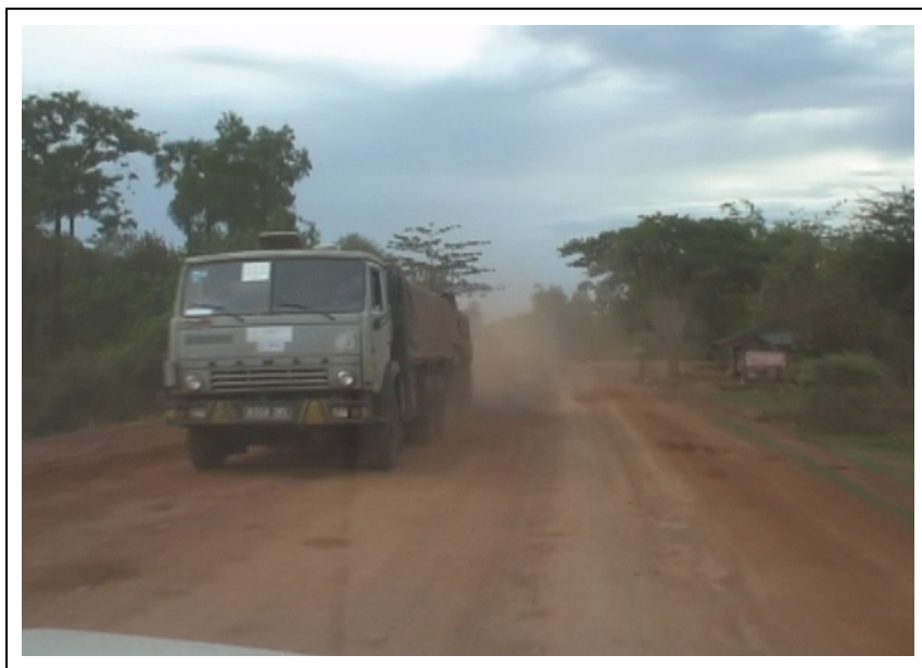
Figure 14 Dust clouds created by vehicle passage in dry season can adversely affect visibility: driver would not have a clear view of any overtaking vehicle.
