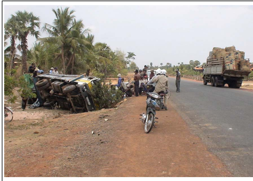
Figure 13 Deep irregularities in sideslope can cause vehicles to roll over if they veer off the carriageway.
