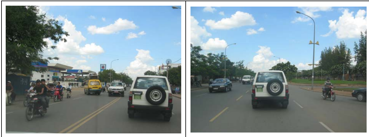
Figure 26 Yellow van and motorcycle causing problems and potential danger by corner-cutting when making a left turn.
