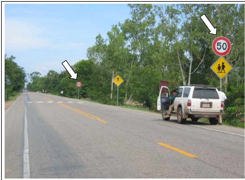
Figure 11 Lower 50m speed limit for zebra crossing – applied over only 80m length of road.
