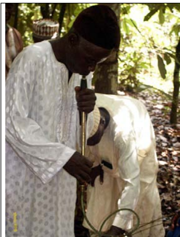
Priming a trombone sprayer prior to application, Nigeria, photo by R. Bateman
