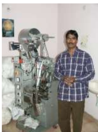
Company 2. Semi-automated bagging machine for pheromone lures.
