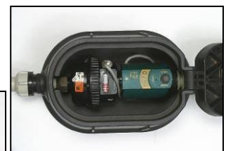
Volumetric Controllers RWE Thames Photos < ↑
