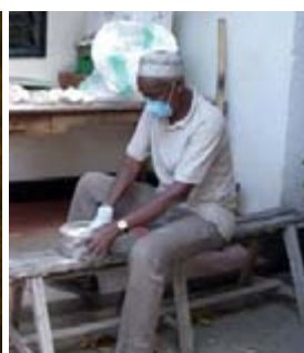
Sieving (100um aperture) of ground diatomite prior to drying to produce local DE
