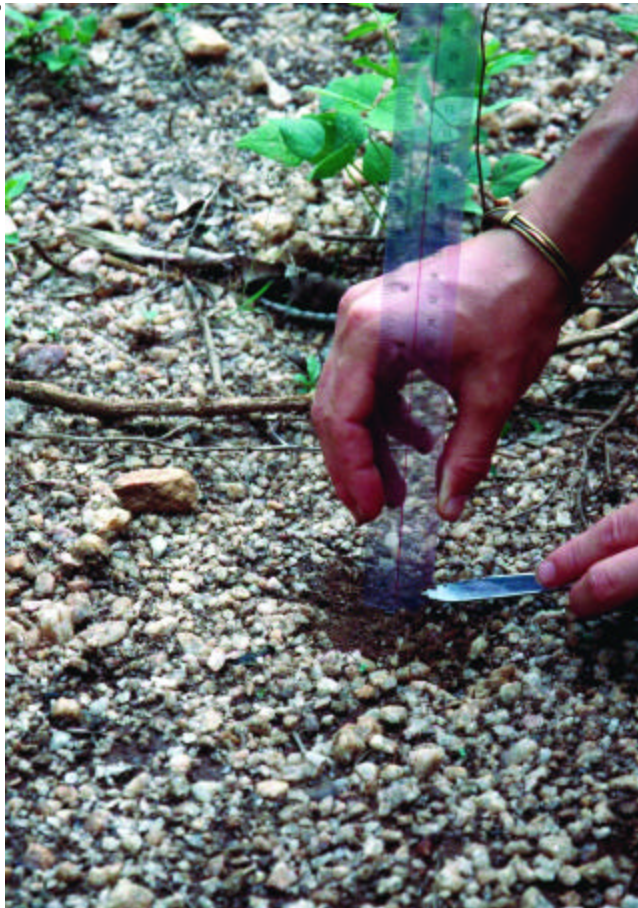
Figure 11.3: Detailed view of assessment of depth of armour layer
