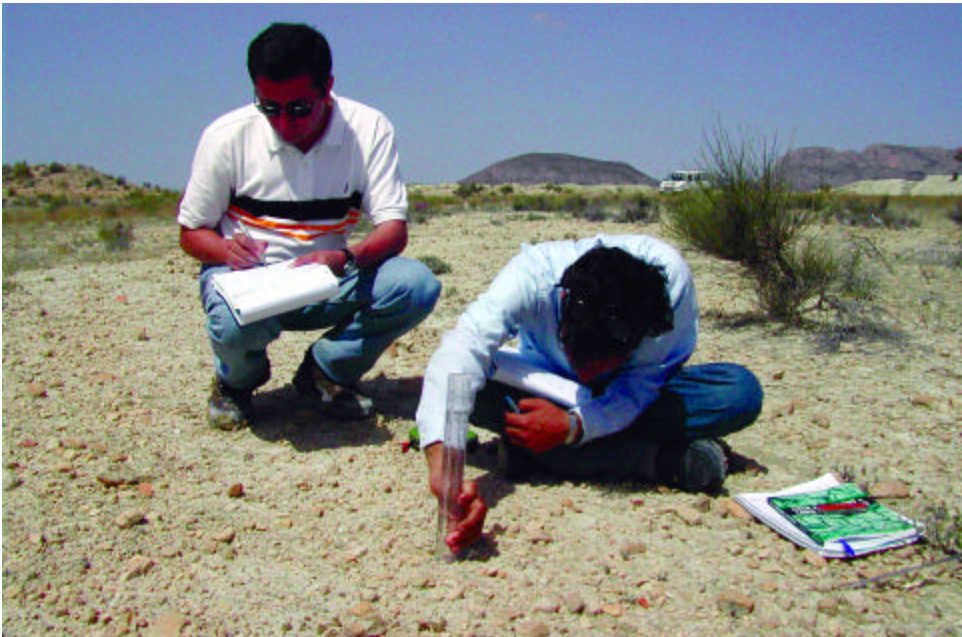
Figure 11.2: Measuring an armour layer in the field with farmer and researcher
