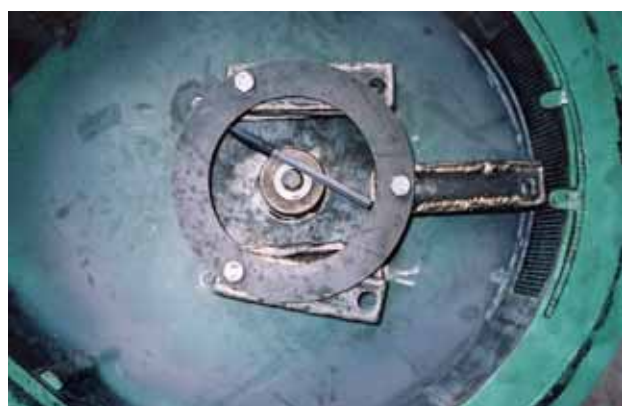
Plate 22 Close up of modified TD Hammer Mill beaters
