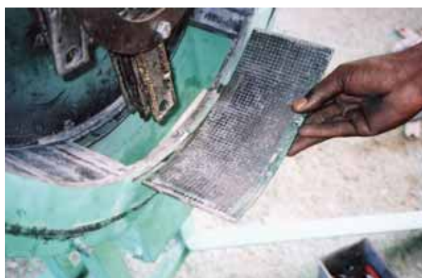
Plate 23 Close up of modified TD Hammer Mill beaters
