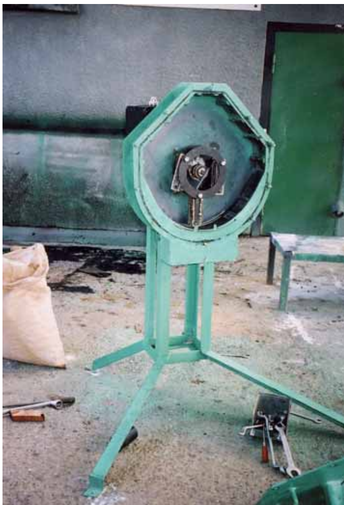
Plate 21 Interior of modified TD Hammer Mill
