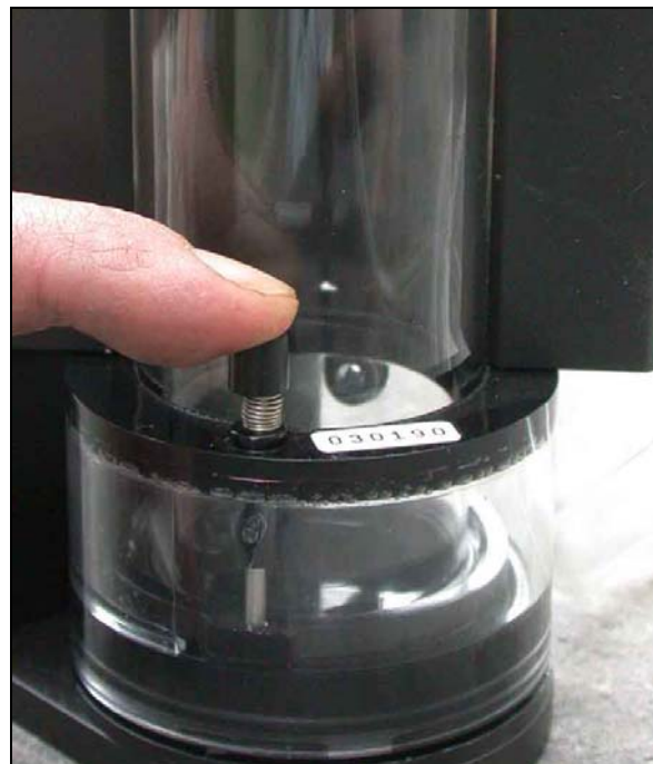
Figure 3: tube to cyclone connects to upper outlet of calibrator
