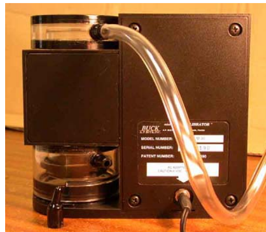
Figure 3: tube to cyclone connects to upper outlet of calibrator
