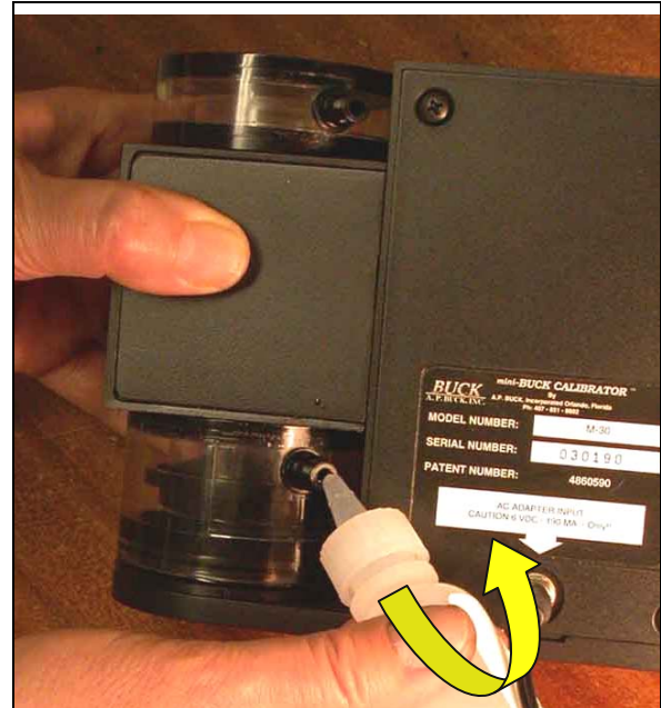
Fig 1: Placing a few drops of soap solution into the bubble chamber through the lower opening
