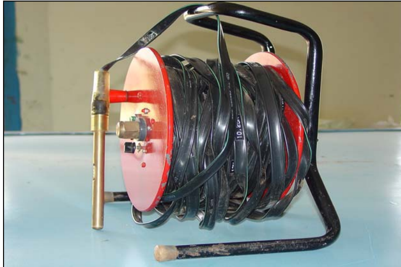
Ground water level measuring device
