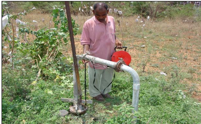
Farmers measuring level of ground water through measuring device
