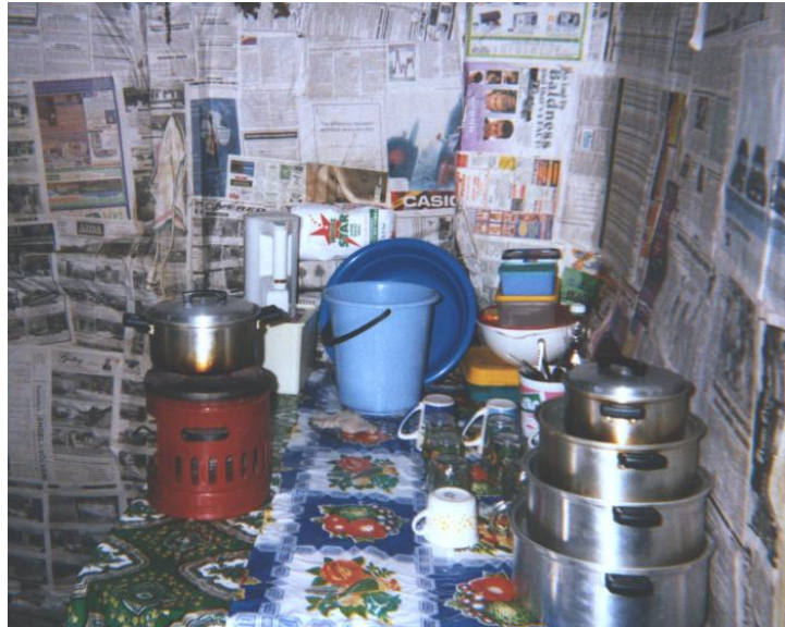
Figure 8 Cardboard and newspaper (for insulation) combine with kerosene stoves to create fire risks
