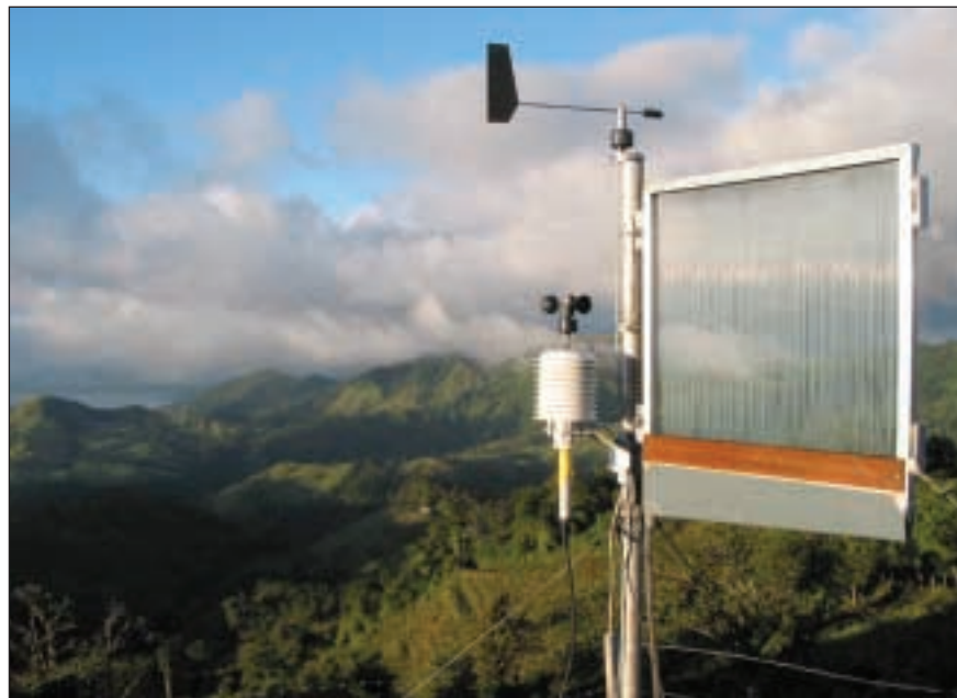
Plate 16) A "harp" type rain gauge for measuring fog and mist in the Rio Chiquito catchment, Costa Rica. © Arnoud Frumau
