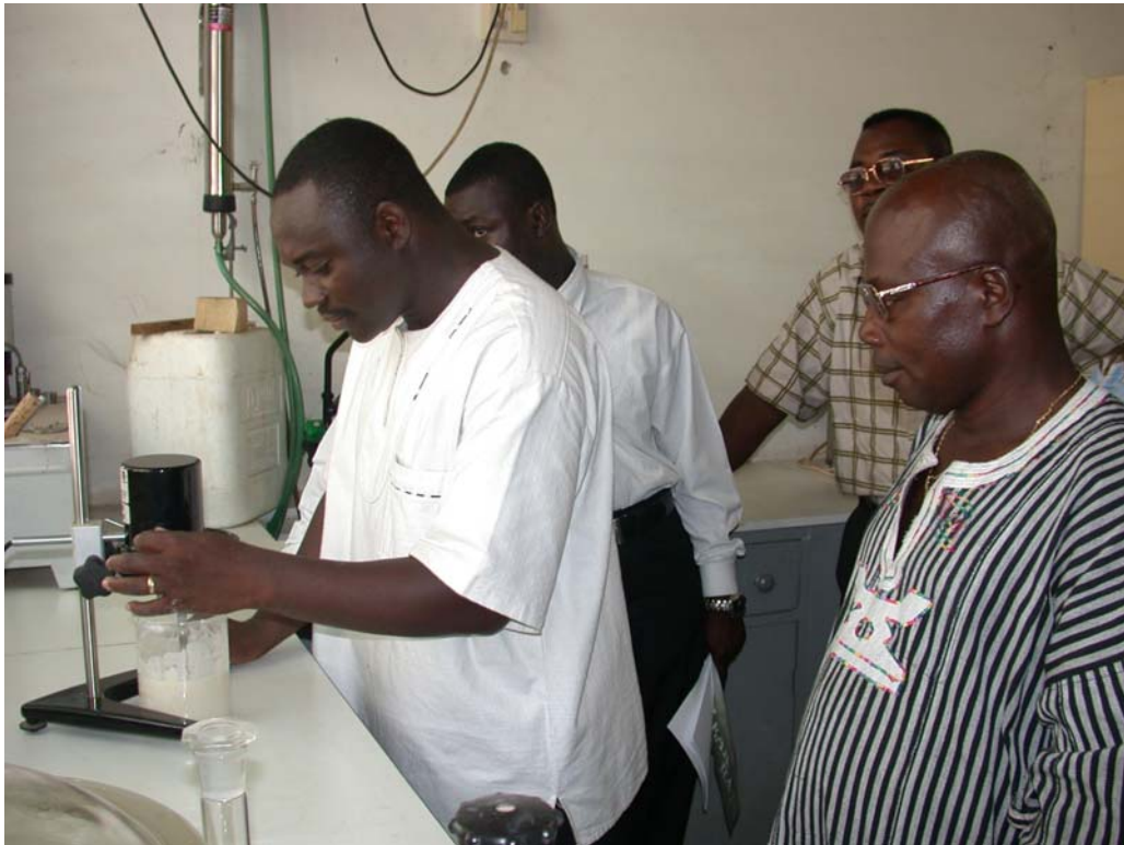
Resource person formulating plywood adhesive with cassava flour as extender.
