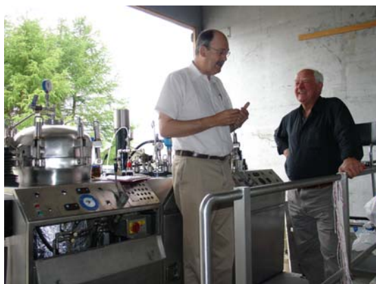
A compact semi-continuous extraction facility using HFC-134a. (Peter Wilde Associates Ltd.)
