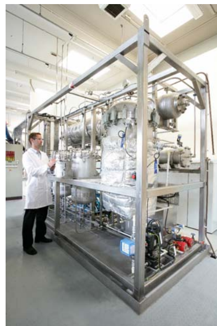
Pilot plant for semi-continuous extraction using HFC-134a at Ineos Fluor Ltd.
