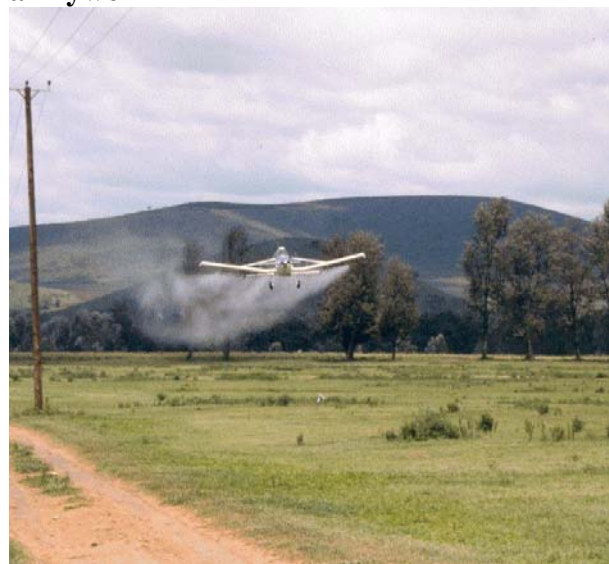
Plate 12 Aerial application of NPV to armyworm
