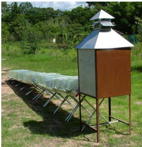
Figure 25. Drying tower with heating funnel
