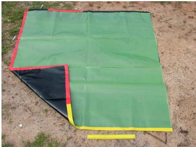
Figure 31. A large sterilization bag, folded at one corner to show the black plastic under surface, the upper surface was made of heavy duty UV resistant clear plastic.
