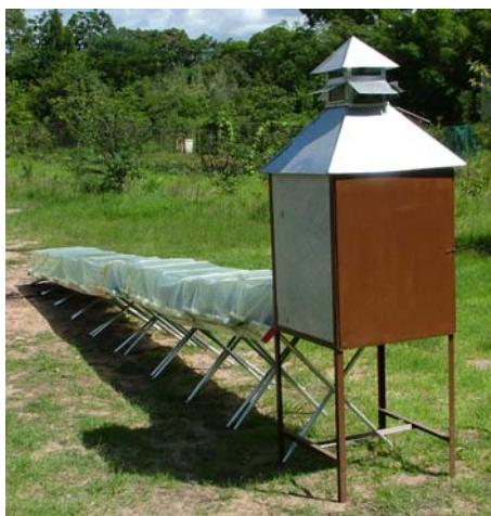
Figure 25. Drying tower with heating funnel
