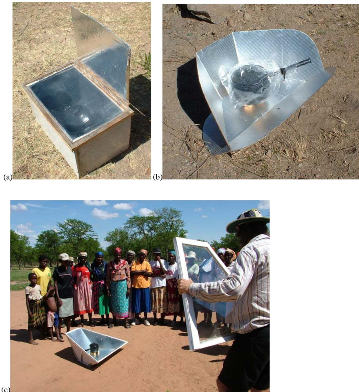
Figure 21. The various types of solar cookers a) the black box with a reflector b) a cardboard cooker coated with a silver film on the inside and c) a sheet metal cooker being demonstrated to the women from surrounding households at Kapeni.
