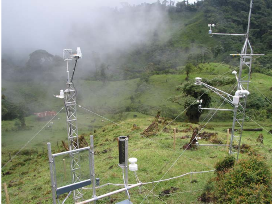
Figure 6f. Micro-meteorological equipment as used at the San Gerardo pasture site.
