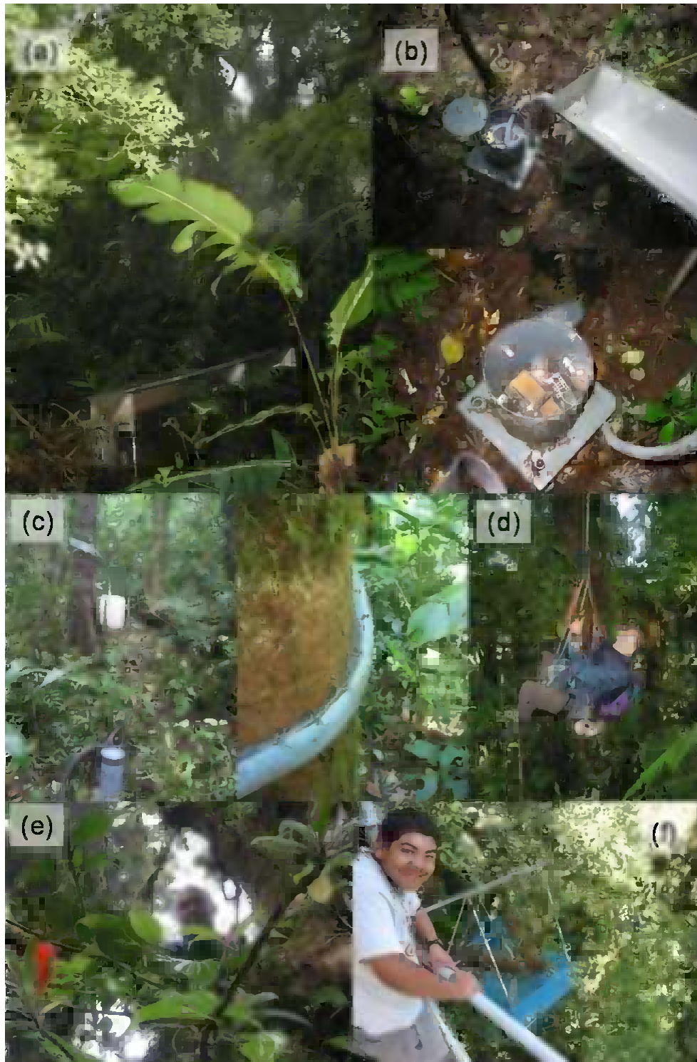
Figure 5. Approaches to net precipitation and bryophyte fog interception behaviour: (a) Throughfall trough overview. (b) Detail of throughfall trough tipping bucket system. (c) Stemflow set-up. Note manual throughfall gauge in foreground in left-hand panel. (d) Access to the canopy for moss biomass determinations through single-rope climbing techniques. (e) Epiphyte and moss specialist Dr Lars Koehler sampling mosses high up in the canopy. (f) Field assistant Eder Morales during a within-canopy moss drying experiment at the forest tower site.
