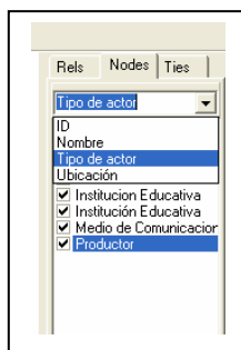
Go to Nodes in the window on the right-hand side of the screen (Figure 25) where the different agrupations of the actors according to their attributes. For this example we chose “Producers”.
