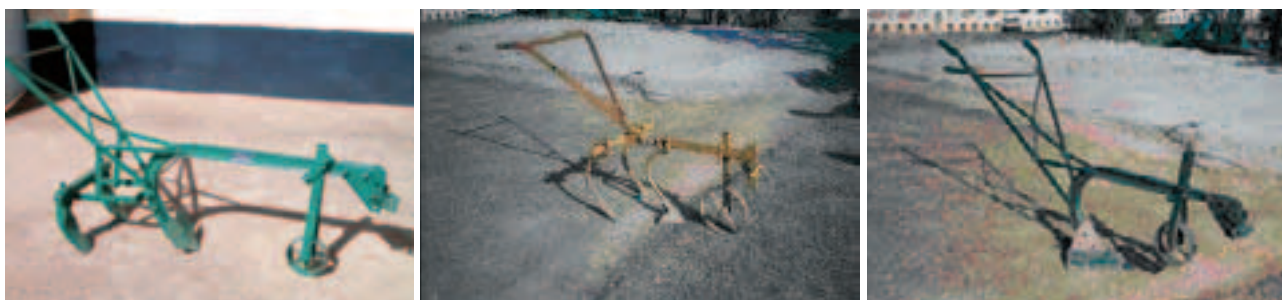
Left to right: SAARI weeder; SG2000 weeder (from Kenya); plough minus mouldboard
