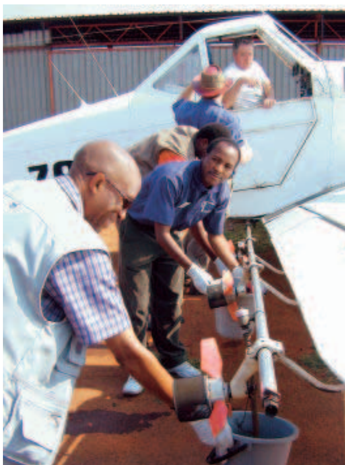
Calibrating the aircraft prior to spraying operations during the September 2005 training course
