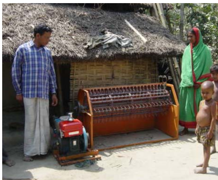
Fig. 20. Ruhul Amin showing his open drum thresher and diesel engine
