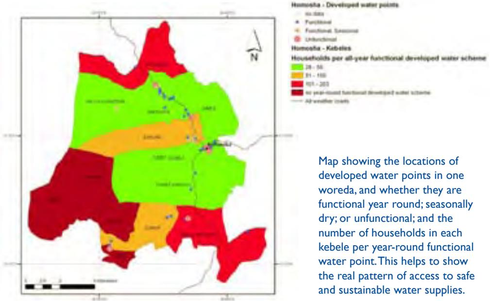
Map showing the locations of developed water points in one woreda, and whether they are functional year round; or unfunctional; and the number of households in each kebele per year-round functional water point. This helps to show the real pattern of access to safe and sustainable water supplies.
