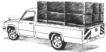
Above: Once the straw has been baled, the same truck can carry 260 kg (100 kg more)
