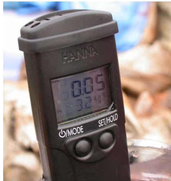
RIGHT: The meter shows a reading of 0.05 mS/cm, almost devoid of nutrients
