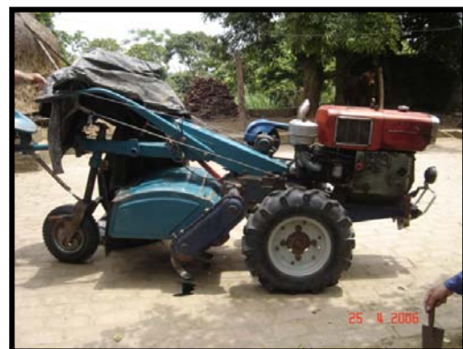
Plate 5 Agricultural rotavator that may be used for mixing lime or cement stabiliser
