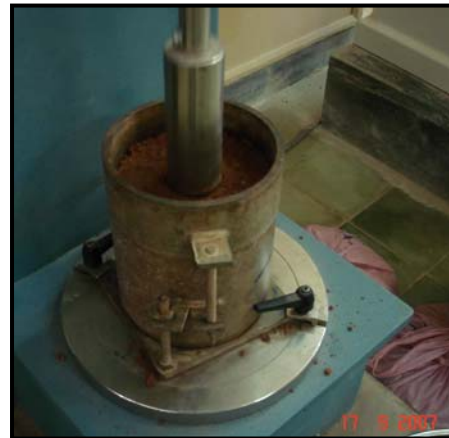
Plate 4 CBR Strength Testing
