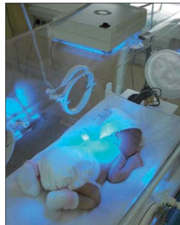
The University of the Republic, in Uruguay, developed 'Bililed' – a lamp for treating severe jaundice in newborn babies. Jaundice is treated using a very precise source of blue light which helps to avoid the toxic effect of the 'bilirubin' molecules that cause it. Commercially-available lamps, based on digital technology – light emitting diodes (LEDs) – are costly, because each LED has very little power and thousands of them are used for the required intensity. Bililed uses fewer LEDs and is therefore cheaper. By substituting LEDs with a system of light concentration, they got the same effect. Bililed has been installed in several public hospitals in Uruguay, bringing state-of-the-art technology within the reach of public health. ©Hospital Pereira Rossell, Uruguay, 2007
