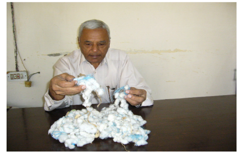
A ginner showing polypropylene trash (blue) in seed cotton.
