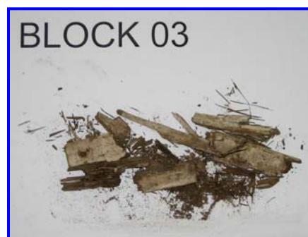
Plate 2: Disintegrated Bamboo from Sample
